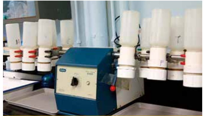
Varroa shaker set up to process. Up to 12 samples are shaken for 30 minutes to dislodge any varroa mites. The mites are then counted and a mite load is calculated. Photo courtesy of the Bee Informed Partnership, Inc.
